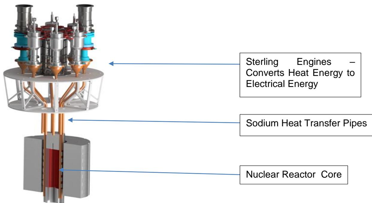
**Figure 1 : NASA 1 kW Prototype Nuclear Reactor of Height 1,9m**
